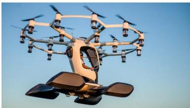
The aircraft, named Hexa™, resembles a large drone with 18 sets of propellers, motors and batteries. It has one seat for the pilot and weighs only 432 lbs – which qualifies it as a Powered Ultralight by the FAA so **no pilot's license is required to fly**. The flight computer is keeping the aircraft stabilized, and the pilot merely provides control inputs using a joystick."
