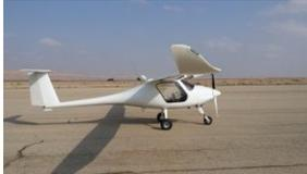
[Uavos](#) has announced that the company has created an unmanned aerial vehicle (UAV) based on the Sinus light aircraft manufactured on a large scale by Pipistrel. This project is a part of an overall plan to create **a multifunctional aerial robotic system that is able to carry out group missions with an integrated special payload.** Test flights demonstrated excellent synchronization of the on-board control system with payloads during a simultaneous flight of three unmanned vehicles.
