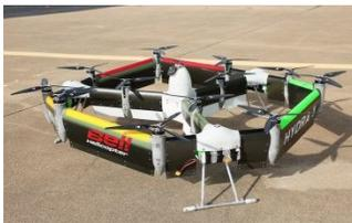
The distributed-propulsion Hydra has 12 foldable propellers mounted on the wing and spokes. The tailsitting VTOL Hydra transitions to horizontal flight for increased efficiency.
