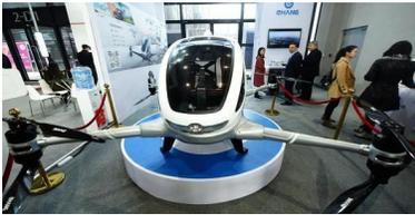
The electricity-powered drone, called EHang 184, can carry up to 220 pounds (100 kilograms) of weight for 25 minutes. It has an average cruising speed of 37 miles per hour (60 kilometers per hour) and has a ceiling of 500 meters above sea level.
