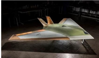
*The Magma drone is controlled by blasts of air taken from its jet engine and blown over its wings*
