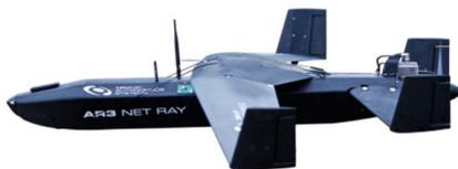
Going by the slightly laboured acronym [FLAIR](#) (FLYing ultra-broadband single-shot Infra-Red Sensor), the fixed-wing drone will be able to reach speeds of 120km/h, an altitude of 4,000m, and cover a radius of 80km. Onboard will be a super-continuum **laser** capable of detecting tiny concentrations of **a range of gases, including carbon dioxide, methane, sulphur oxides, and nitrogen dioxide.**
