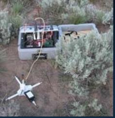
Integrated electric and magnetic field sensor for subsurface mapping in field use. *Credit: QUASAR Federal Systems, Inc.*
