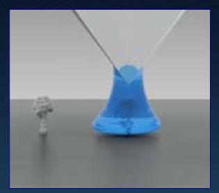
Dip Pen Nanolithography for nanofabrication. *Credit: Nanolnk*
