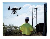
Phoenix Air Unmanned, LLC (PAU) received a broad area waiver from the Federal Aviation Administration authorizing utility powerline inspection flights beyond the visual line of sight (BVLOS) of the remote pilot in command. The authorization spans powerline infrastructure across the United States and builds upon thousands of miles of BVLOS transmission line inspection flight experience.
