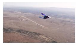
The flight's objectives included evaluating the performance of the spaceship in the glide phase, following the modification period. The team were also able to continue evaluating the handling qualities and flight controls of the spaceship, and gather data on the new mothership pylon with the spaceship attached during standard climb and release.
