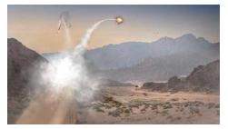
During a Department of Defense-led exercise at Yuma Proving Ground, Arizona, the 70mm APKWS-guided rockets demonstrated 100% effectiveness when fired against 25-to-50-pound drones traveling at over 100 miles per hour. The APKWS<sup>®</sup> C-UAS solution is platform agnostic, permitting multiple options to accelerate
