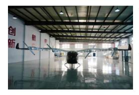
The M1 is a 4,400-lb. gross-weight lift-plus-cruise eVTOL aircraft with a wingspan of 49 ft. The vehicle has four wing booms carrying 16 lift rotors for vertical flight and four propellers for wing-borne cruise flight. The tail connects the booms to the rear fuselage. The aircraft has a maximum payload of 500 kg and a 124 ft<sup>3</sup> flat-floor cabin that can accommodate 32 standard postal boxes, Vertaxi says.
