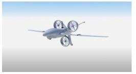
Ancillary is an X-plane program to demonstrate a shipbased long-endurance VTOL unmanned aircraft.
