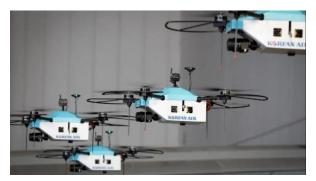
The airline says it has developed technology that for the first time allows a swarm of drones to inspect an aircraft exterior. Last week it demonstrated the concept on one of its aircraft inside a hangar in Seoul. Four unmanned aerial vehicles have been programmed to simultaneously take photos of preplanned areas.
