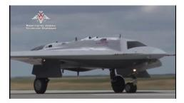
Designed by UAC subsidiary Sukhoi, the S-70 prototype first took off in August 2019. The UAV is designed to carry a payload of 13,200lb, have a flight range of 3,240nm and an operating ceiling of 59,000ft. The aircraft is capable of carrying air-to-air missiles and reconnaissance equipment.
