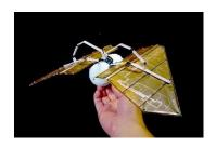
Aerobat's design is based on bat wings, collapsing and expanding to maximize lift generation and avoiding powerful air jets like rotorcraft do. A bat wing has 40 joints, and the Aerobat makers tried to replicate that. Like bats, a single wingbeat is composed of a downstroke phase, where the drone's wings are extended and swing down, and an upstroke phase, where the wings are
