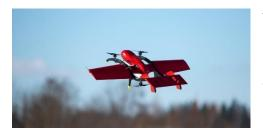
The FIXAR 007 (named for its 7-kilogram weight) utilizes a unique design. As opposed to many conventional fixed-wing VTOLs, it does not require the angle of its rotors transition for forward flight. It uses Fixed Angled Rotors, which is how the aircraft (and the company) derives its name. Nor does it require separate motors for vertical
