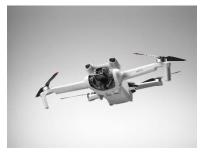
DJI Mini 3's Intelligent Flight Battery grants it a max flight time of up to 38 minutes, which can be extended by up to 51 minutes with the Intelligent Flight Battery Plus. DJI O2 digital video transmission provides a 720p/30fps live feed from up to 10 km away, with anti-interference technology guaranteeing a stable image connection throughout the flight. Mini 3 has a wind resistance at up to 10.7 m/s, allowing it to hover. DJI Mini 3 also
