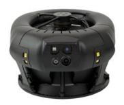
Based on Cleo's Dronut, the TacDronut is a rugged portable sUAS that suits the needs of Soldiers requiring a drone capable of operating within enclosed spaces. Capable of enduring impact without taking damage and operating in both GPS enabled and GPS denied environments, the Dronut features a highly capable and adaptable onboard intelligence and sensor payload. Following the prototype's successful demonstration with the 82nd Airborne
