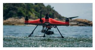
SwellPro has a very niche line of waterproof drone products and accessories. The company says they can be used for research, recreation, and even fishing, providing you purchase an optional bait-dropping release mechanism with a whopping 2-kilogram payload capacity. That means you could lift a baited line with a heavy
