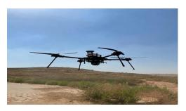
NavGuard is a real-time optical navigation system that enables seamless and accurate autonomous GNSS-free navigation for tactical UAS platforms in areas where the GNSS signal is spoofed, jammed, or simply unavailable. Using machine vision technology, AI, advanced optics, and sensor fusion, NavGuard can be installed on different unmanned aerial platforms to enable safe and
