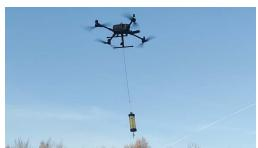
SPH Engineering introduces the Remote Water Sampling System, a new UAV-based solution within UgCS Integrated Systems product line. The trial flight was conducted at a Latvian lake to proceed with water sampling for subsequent analysis in a laboratory.
