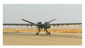
General Atomics' aeronautical systems has introduced an unmanned aircraft system that offers short-takeoff and landing capabilities and can carry up to 16 Hellfire missiles in support of armed reconnaissance, attack and armed overwatch missions.
