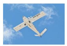
Singular Aircraft is exploring two sizes of Flyox drone. The smaller version will have an internal capacity of 3,400 pounds, with a two-hour flight time and a range of 260 miles. The larger drone, owing to its greater fuel capacity, will only carry 3,000 pounds internally, but can operate for four-and-a-half hours, and reach distances of over 500 miles. Carrillo says the Flyox
