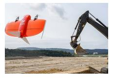
WingtraOne takes-off and lands as a multicopter but flies in the air as a fixed wing aircraft. This technology eliminates the risk of damaging the aircraft while landing, lets the drone carry professional sensors and still allows mapping of large areas. The PPK (post process kinematics) upgrade allows the aircraft to reach new level of accuracy down to 1 cm without any ground control points.
