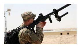
A 1st Security Forces Assistance Brigade (SFAB) Soldier uses a Drone Defender to capture and control a drone as its flying. It uses an electromagnetic pulse to disable its target and has a range of 600 meters.
