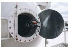
Flyability's Elios series offers a unique and sophisticated solution to the problem of using drones in small, dark and difficult spaces. The innovative cage around the drone allows pilots to navigate narrow areas like the insides of mines, girders, ship hulls and more.
