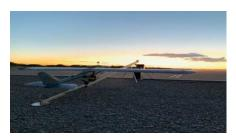
Silent Falcon™ UAS Technologies (SFUAS), an Albuquerque-based service provider and original equipment manufacturer announced that the Silent Falcon E1 UAV has completed 500 hours of successful flight testing and operations. It is a solar electric, fixed wing, Unmanned Aircraft System. It is noise-free, emission-free, and provides long-range, low-cost ISR
