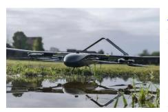
FlyDragon Drone Tech has detailed the specific design features of the FDG30 Mako Shark that help enable the VTOL UAV to achieve ultra-long endurance flights of six hours. Designed for aerial surveying and surveillance applications, the electric UAV combines the launch and landing advantages of a multirotor with the endurance of fixed-wing aircraft.
