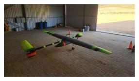
While there is still a way to go until the Dragonfly V is fully ready for production, the aircraft has already demonstrated remarkable handling and efficiency during its first flights. Dragonfly V is a fixed-wing STOL (Short Take-Off and Landing) drone that is targeted for use in multi-mission applications in landscape management such as agricultural pest
