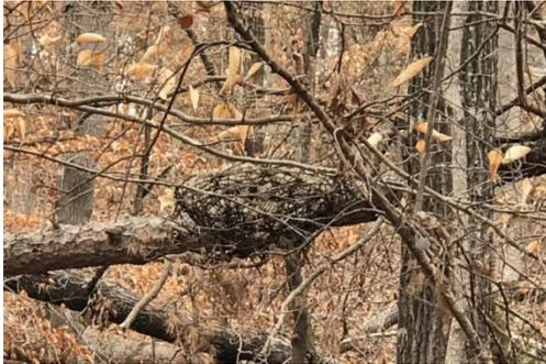
*A "bird's nest," developed by Clemson University landscape architects, houses and hides the electrical components of the drone detection system.*
