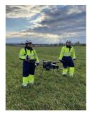
Sandnes, Norway – Nordic Unmanned AS has carried out a successful test flight with a hydrogen fuel cell powered Staaker BG-200. It is equipped with a 2kW customized fuel cell system from HES and a
