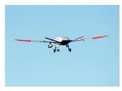
Taking off from the company's test site at the MidAmerica Airport in Illinois near St. Louis, Mo., the Stingray prototype flew for two and a half hours with an aerial refueling store (ARS) slung under its wing.
