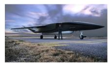
Alabama-based Aevum Inc.'s Ravn X drone plans to offer the U.S. Space Force and other customers launches to Low-Earth Orbit within three hours of tasking. The 80-foot, 55,000-pound drone with a wingspan of 60 feet is to have second and third stages that will carry payloads up to 500 kg. to LEO.
