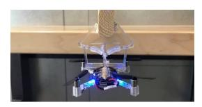
Engineers at Colorado State University have equipped a tiny drone with a mechanical gripper that allows it to hold onto objects using less power and producing much less noise.
