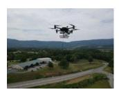
Zenith AeroTech has flown it's heavy lift tethered drone, the Quad 8 multi-rotor, for more than 108 hours of continuous flight.
