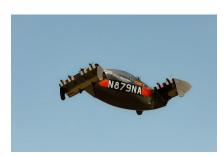
Opener's BlackFly during a test flight. Engineers have spent a decade nurturing this new breed of aircraft, electric vehicles that can take off and land without a runway.
