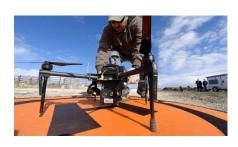
A DJI Matrice drone equipped with a thermal imaging camera is prepped for takeoff at a research feedlot in Texas.
