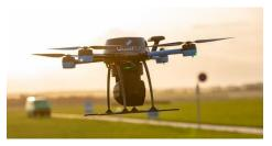
Danish startup QuadSAT uses specially equipped quadcopter drones as satellite stand-ins to help antenna makers and their customers test and calibrate.
