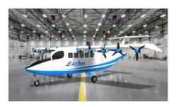
Airflow has two eSTOL aircraft variations, a Model 100 and Model 200. Airflow's Model 100 can carry four passengers or 800 lbs of cargo, only needs 150 feet to take off, and has a 250-mile range. The company's Model 200 has a nine-passenger or 2,000 lb cargo payload, needs 250 feet to take off, and has a 500-mile range. Both aircraft are 100 percent carbon neutral.
