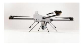
The <u>C100</u> is a man-packable heavy-lift quadcopter platform that holds the world record for the longest-endurance battery-powered sUAS. Capable of <u>80 minutes</u> of flight with payload, the low-SWaP (size, weight, and power) autonomous UAV folds into a small rucksack and can be deployed and airborne in under 2 minutes.
