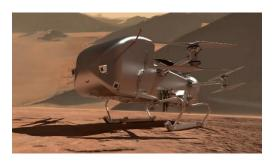
Dragonfly will be equipped with cameras, a chemical lab and a nuclear-powered generator. The helicopter has drills in its landing skids for collecting samples from the surface.
