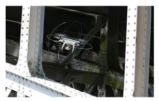
Team UAV has launched a new collision tolerant Dronecage to make confined space inspections and surveys more cost effective, higher quality, and available to all operators.
