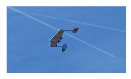
Whisper's ultraquiet 55-lb. ISR drone has a single top-mounted 10-lb.-thrust electric ducted fan.
