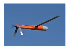
Air launched effects are a form of unmanned air vehicle that the US Army envisions launching from aircraft, in particular its Future Attack Reconnaissance Aircraft and its MQ-1C Gray Eagle UAV. The service wants to use the UAVs for multiple missions behind enemy lines, including intelligence, surveillance and reconnaissance, electronic warfare and loitering munition strikes.
