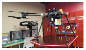
Honeywell Aerospace is currently working on version 2 of its IntuVue RDR-84K radar system, which can be seen mounted on the drone
