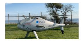
The European Maritime Safety Agency has kicked off a large-scale emissions monitoring campaign in the Baltic Sea this week. As part of the project, drones are being deployed through Germany to remotely measure the sulfur content in ships' exhaust plumes and detect violations of the applicable limits.
