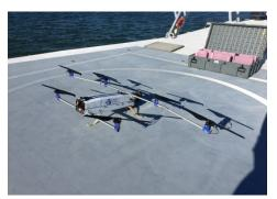
Several US Navy organizations observed as we conducted maritime operations and demonstration flights with this new UAS with impressive range and payload capabilities. HAMR has multiple government and commercial applications – based on three-hour maximum endurance, seven-pound maximum payload, or combinations in between. <a href="http://oncourse-llc.com/aac-hamr-flight-demo-aboard-us-navy-m80-stiletto/">http://oncourse-llc.com/aac-hamr-flight-demo-aboard-us-navy-m80-stiletto/</a>
