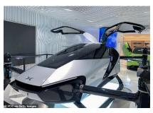
Cruise Speed: 100 mph. Range: 110 miles. Max Flight Time: 1 Hour
