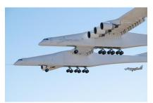
The Mojave, California-based company plans to use its massive, six-engined Roc aircraft as a launch platform for hypersonic vehicles and missiles. The aircraft, which has a record-setting wingspan of 117m (385ft), was developed by Scaled Composites to air-launch rockets into orbit.
