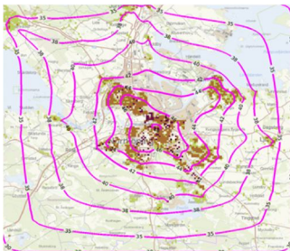
Image: Noise footprint over Norrköping municipality, overlaid with the population density grid
