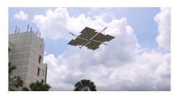
Engineering students from the National University of Singapore developed a quadcopter that can fly solely on solar energy. The 5.73-pound prototype has flown over 32 feet with 148 silicon solar cells and a carbon fiber frame that takes up about 43 square feet. Solar-powered quadcopters have been spotted before, but the UAV that
