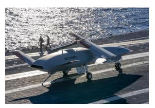
Boeing's MQ-25 Stingray unmanned aerial refueler has successfully completed its first sea tests with the U.S Navy aboard the USS George H.W. Bush aircraft carrier. The tests were also the first conducted on a carrier for the MQ-25 and covered deck handling maneuvers including taxiing on the deck, connecting to the catapult, clearing the landing area, and parking on the deck.
