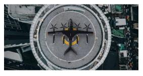
Vertical Aerospace's VX4 eVTOL aircraft will carry four passengers around 100 miles at speeds of 200 mph.
