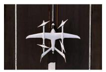
ALIA is a distributed, direct-drive electric propulsion system with eight lifting motors used for vertical lift and two internal motors used for cruising
