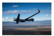
General Atomics Aeronautical Systems has successfully flown an MQ-9A UAS north through Canadian airspace past the 78th parallel, proving the platform's ability to fly in high-latitude environments. The aircraft was deployed in its "Big Wing" configuration, which features a 79-foot wingspan, an endurance of over 43 hours, top speeds of 220 KTAS, and a
