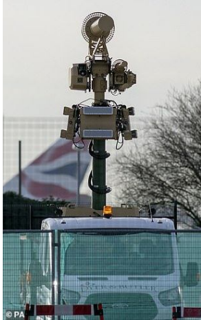
The Anti-UAV Defence System is able to detect, track and ground drones
