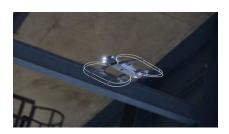
ROBi is equipped with different sensors and camera systems. For example, during the interior inspection of a large tank, we discover a possibly defective weld seam. We can then replace the camera system with a system that measures the thickness of the coating or takes a sample to tell how serious the damage is. A complete inspection of a large tank can
