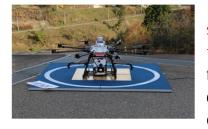
This system enables a drone to safely fly beyond visual line of sight (BVLOS) and remain in contact with the operator at all times. That includes being able to transmit a live image of the flight path and its surroundings, allowing the remote operator to control the aircraft by sight. The network connection allows the drone to respond to sudden changes to flight routes and execute
