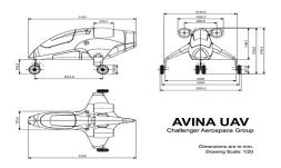
The Avina soft wing unmanned aircraft is powered by two EDF fan units with power from a hybrid power generator, top speed of 130 km/h. The Avina will be one of the most versatile systems on the market, to embark a great variety of mission-specific modules: cameras, IR sensors, droppable cargo or even a human pilot for particularly sensitive missions.
