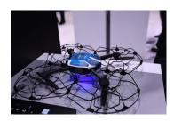
The drone is designed to fly safely indoors where GPS may or may not be available. Additionally, the device has over 4 billion unique color combinations for aerial displays that are aided by an Intel Indoor Location System for navigating inside a closed space. Think complicated light patterns in the air for a general idea of the capabilities of this system. <a href="https://www.wetalkuav.com/intel-drones-">https://www.wetalkuav.com/intel-drones-</a>
