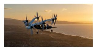
EASA has published what it claims are the world's first proposed noise certification standards for eVTOLs. Known as the Environmental Protection Technical Specifications (EPTS), the proposed specification would be applicable to eVTOLs powered by multiple vertical, non-tilting, evenly distributed rotors.
