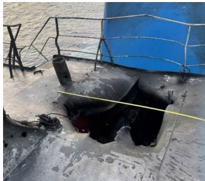
Damage caused by a drone attack July 29 on the oil tanker Mercer Street off Oman.
