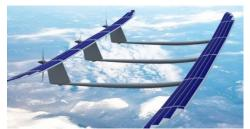
A high-altitude unmanned-aerial-vehicle prototype, powered by solar panels and batteries, performs functions commonly attributed to spacecraft flying in low Earth orbits.
