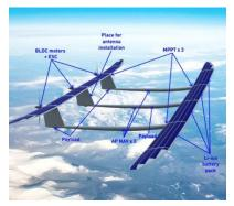
Various combinations of composite materials are used in the wing design. The sets of solar panels are divided into groups located in relatively equal planes of the wing, due to the uneven illumination of the wing in flight, and to obtain the maximum efficiency factor. The power circuit of the aircraft has two to four maximum-power-point-tracking (MPPT) converters of solar energy. Telemetry data obtained from them (power, voltage, current, and temperature), as well as from other
