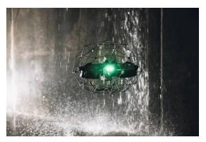
Flyability has unveiled the Elios 3, which the company claims is the world's first collision-tolerant drone equipped with a LiDAR sensor for indoor 3D mapping. A new SLAM engine called FlyAware lets it create 3D models as it flies.
