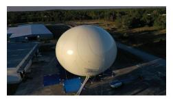
Han Tang Technology/UAV Corp through its subsidiary Skyborne Technology, Inc. has successfully conducted an inflation test of the new DATT SA-70 semi-rigid Airship with drone package.
