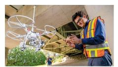
ARMANDO TURA/UNIVERSITY OF VICTORIA — Founders of Niricson, a Victoria, B.C.-based technology company, have developed a novel drone-based collection and damage-assessment software system to inspect and detect problems with aging infrastructure.
