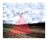
Detection and Ranging) technology has become an important tool for the surveying industry and is used to perform 'laser scanning' and generate 3D point cloud images.
