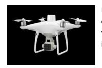
P4 Multispectral features a gimbal-stabilized imaging system composed of one RGB camera and a multispectral camera array with five narrow band sensors – including red edge and near infrared – that are capable of capturing visible and invisible light.
