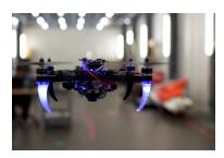
Developing a system that's both easy to use and self-contained is quite a challenge, but roboticists from the University of Pennsylvania, U.S. Army Research Laboratory, and New York University are up to it—with just a pair of lightweight gazetracking glasses and a small computing unit, a small drone will fly wherever you look.
