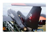
Airbus has successfully carried out manned-unmanned teaming test flight campaigns for future air combat systems. The campaigns were conducted using five Airbus-built Do-DT25 target drones that demonstrated the ability to control unmanned systems from a manned aircraft.
