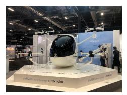
While the current full-scale prototype has been made for one (1) passenger traveling at 90 km/h (56 mph) for a range of 15 km (9 miles), Tecnalia says the aircraft can be scaled up for a four-passenger aircraft at 190 km/h (118 mph). The aircraft has four sets of propellers powered by electric motors which are located on the four corners of the aircraft. Each propeller has its own electric engine which makes for a total of sixteen propellers and electric
