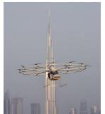
The flying taxi developed by German drone firm Volocopter resembles a small, two-seater helicopter cabin topped by a wide hoop studded with 18 propellers. Meant to fly without remote control guidance and with a maximum flight duration of 30 minutes, it comes with plenty of fail-safes in case of trouble: back-up batteries, rotors and, for a worst case scenario, a couple of parachutes.
