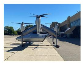
ASX's Sigma Six has six rotors on a tilting wing, interchangeable payload modules and an automated ground vehicle to handle them.
