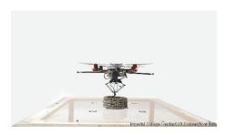
Writing in the latest edition of *Nature*, Dr Kovac describes a system of flying robots that is composed of two types of multi-rotor drones: builders and scanners. The builders carry the 3d-printing nozzle. The scanners are robots equipped with cameras that are responsible for monitoring the progress of the builders.
