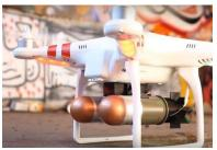
Jane's reports that Canadian counter UAS company AerialX is finalizing the development of DroneBullet, "an intuitive, high-speed multi-rotor kinetic energy interceptor solution designed to counter small multirotor and fixed-wing unmanned aerial system threats."
