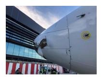
A <u>Boeing investigation</u> — completed at the behest of the National Transportation Safety Board — cleared the hypothetical UAS of any wrongdoing. Engineers determined that no object was the culprit, but that damage was likely the result of pressure differentials during descent.
