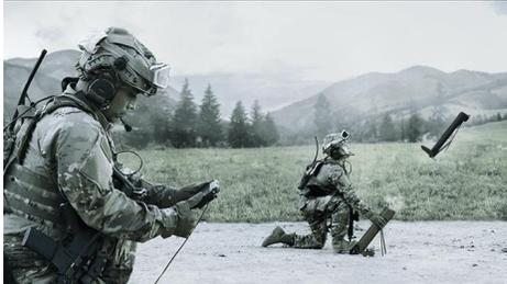
The Switchblade 300 Block 20 is designed to be portable, lightweight, and easy to operate, requiring only a single operator. It features a new tablet-based Fire Control System that allows operators to easily train, plan, and execute missions, while an integrated control directly onto the launcher tube simplifies operation even further.
