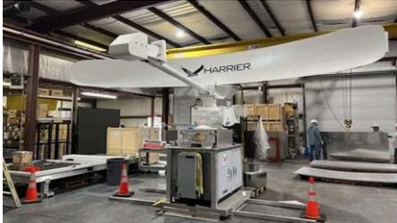
[DeTect](#), Inc. has announced a significant milestone in its radar technology development. The company has successfully produced its largest and longest-range radar to date – the HARRIER BAR300. This extended-range radar is capable of aircraft detection at a range of **30+ nautical miles**.
