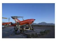
A BQM-34 unmanned aircraft prepares to launch at White Sands Missile Range during the August 2021 test.
